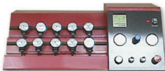
Gauge endurance test machine tests manometers to 30K cycles
